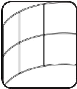
Wave Horizontal Curve frame constructed of 30mm tube. Frame assembles with snap buttons. This is the base frame for all FMLT-2 kits on this page.
