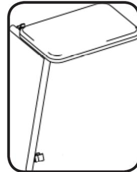
Side mount counter supports are constructed of 30mm brushed tube, 2 clamps and counter top bracket.
