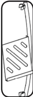
Side mount literature holders constructed of a curved 30mm brushed tube, 2 clamps, & silver powder coated literature holder.
