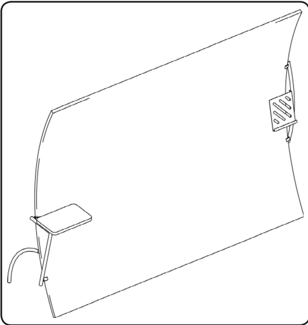
Side counter supports should be attached to side of main frame so that top of support is 39" from ground. Then attach counter top to support with thumb screws.
