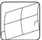
Wave Vertical Curve frame constructed of 30mm tube. Frame assembles with snap buttons. This is the base frame for all FMLT-1 kits on this page.
